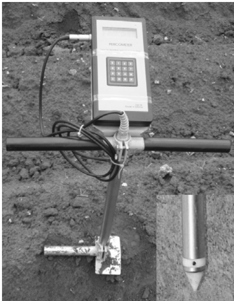
Figure 1. Percometer pressed to the depth 50 cm and the lower end of tube with sensor between conic tip and plastic ring.
